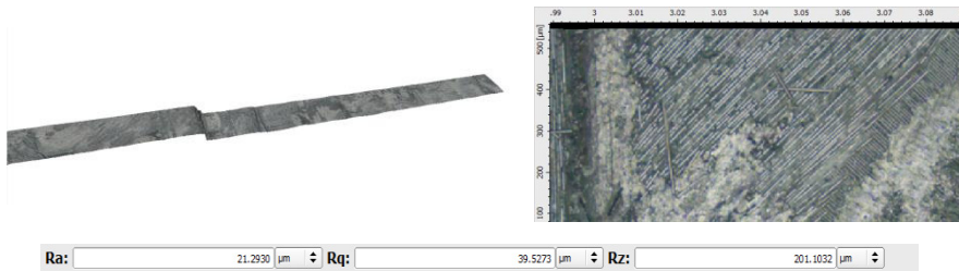
Fig 10. Analyzing surface quality obtained by PCD tool.
