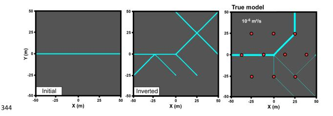
Figure 5: Initial and inverted models for an inversion using drawdown data produced from a true model (on the right) with a homogeneous matrix. The red dots on the true model symbolize the pumping/measurement boreholes for the hydraulic data. The inverted model permits to localize approximatively the karstic network connections but in this case the amount of data is insufficient to have a proper imagery.
