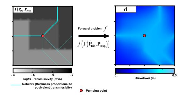
138 <u>Figure 1:</u> Example of a simulated distribution of hydraulic heads (here drawdowns) by solving 139 the forward problem f (Eq.1) for a steady state pumping in a given coupled discrete-140 continuum distributed model  $\Gamma(\mathbf{P}_{\text{Dir}}, \mathbf{P}_{\text{Prop}})$ .
