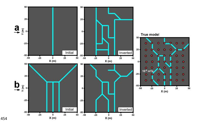
Figure 10: Initial and inverted models for an inversion using drawdown data generated from a true model (on the right) with a homogeneous matrix. The red dots on the true model symbolize the pumping/measurement boreholes for the hydraulic data. A first inverted model (a), starting from a simple initial model, permits to localize approximately the true network geometry. A second inversion (b), starting from a more detailed initial model, permits to produce a more precise network geometry.
