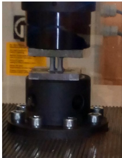
Fig. 6. Position of a sample during a compression test.
