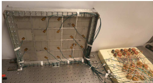
Figure 12: Clamped aluminum plate covered with piezoelectric patches connected to the multi-resonant network.
