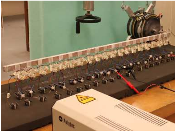
Figure 11. Placement of the shaker and the vibrometer.
