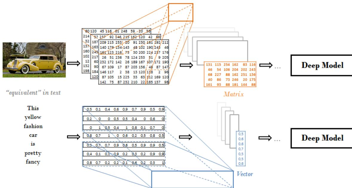
Figure 5: Inside operations of convolution on **Image** vs **Text**. **Image** has real-valued and dense. **Text** has discrete tokens, many artificial and sparse values representation. The output of the first convolution layer on image is still a *Matrix* but on text, it is reduced to a *Vector*.
