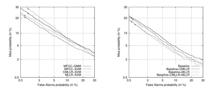
Figure 2: DET curve for the forward individual systems (left, a): MFCC-GMM, MFCC-SVM, CG15/S-SVM and MH12/2t-SVM, and for the baseline and combination systems (right, b). MDC operating points are shown as dots.
