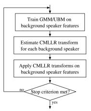
Figure 1: Block diagram for iterative CMLLR GMM/UBM reestimation in the CMLLR/GMM approach.
