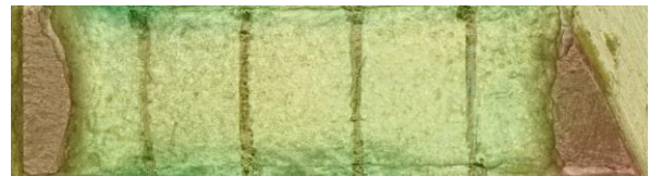
Figure 5. Fracture surface with a central electro-eroded area
