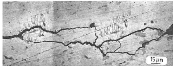
Fig.3b Inter-granular secondary cracks
