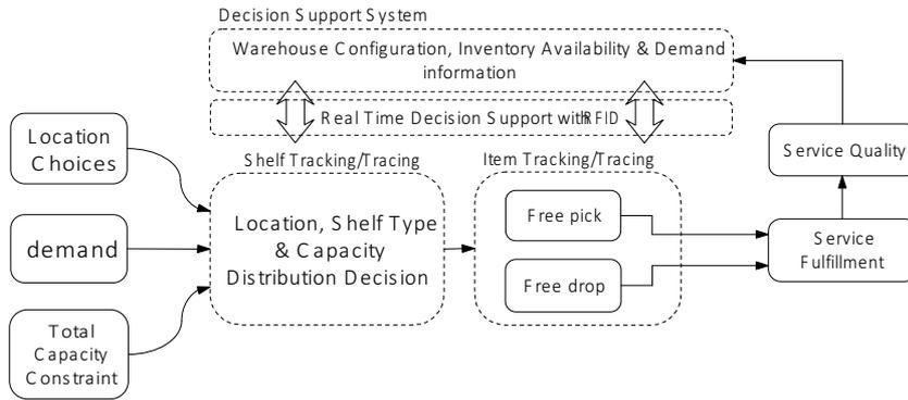
Figure 4: Flexible Warehouse Real-time Decision Support System
