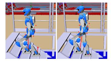
Fig. 6. **Dynamic simulations in Choreonoid:** snapshots at the maximum knee flexion time instant. *Left:* LIP-based pattern generation. *Right:* VHIP-based pattern generation. The former causes HRP-4 to bend its knees more, increasing the risk of shank collision with the staircase. We can also observe the more abrupt CoP transfer of the latter, which is specific to our method.
