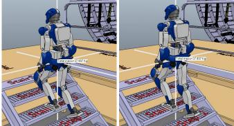
Fig. 7. **Dynamic simulations in V-REP:** snapshots at the toe liftoff time instant. Simulations use the Newton dynamics engine with a time step of 5 ms and one pass per frame. *Left:* LIP-based pattern generation. *Right:* VHIP-based pattern generation. The former causes HRP-4 to bend its knees more, raising the risk of shank collision with the staircase.
