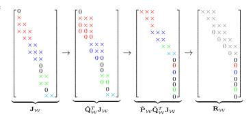
Fig. 12. **QR decomposition for** n = 15 and  $W = \{1, 2, 6, 9, 10, 11, 13, 14\}$ . Cross symbols  $\times$  stand for non-zero elements. Left: block structure of  $J_{W}$ , with one color per block. Middle-left: performing QR decomposition for each block. Middle-right: permuting all zero rows to the bottom. Right: completing the QR decomposition.
