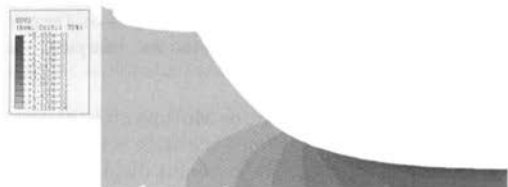
Figure 5. Damage distribution for the AE specimen after the 20 mm displacement cycle.
