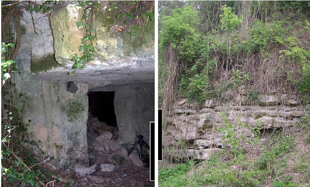
Fig. 3. One of the lateral shift of facies in the Lutetian limestones, the example of the Ditrupa limestones near Fismes. Scale bar about 1 m. Left-hand: in Glennes area, thick homogeneous bank with underground quarry. Right-hand: in Branscourt area, small banks with interbanks = unsuitable for underground quarry.
