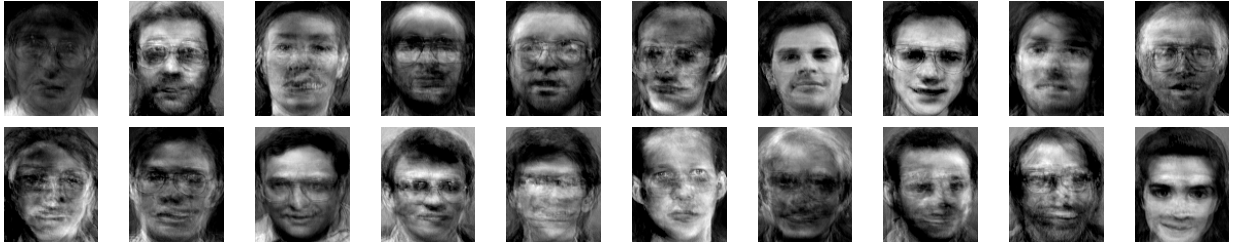
(a) Sparse-NMF basis \{\phi\}_{1 \leq k \leq 20} ( S_w = 0, S_h = 0.6 )
