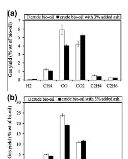
**Fig. 9.** Gas yield of bio-oil pyrolysis at two final temperatures. (a) 550 °C, (b) 1000 °C – effect of ash content.
