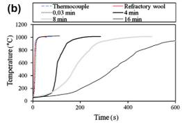
**Fig. 5.** Temperature evolution of the sample during bio-oil pyrolysis in HTR at different heating rates and two final temperatures. (a) 550 °C, (b) 1000 °C.
