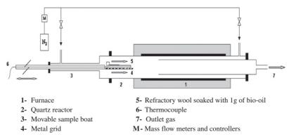
Fig. 1. Horizontal Tubular Reactor (HTR) ready for sample introduction.
