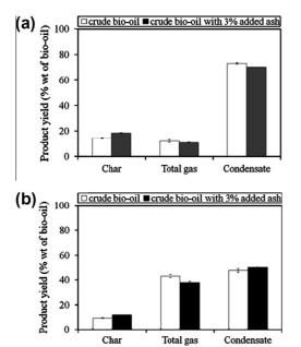
**Fig. 8.** Product yield of bio-oil pyrolysis at two final temperatures. (a)  $550 \, ^{\circ}$ C, (b)  $1000 \, ^{\circ}$ C – effect of ash content.
