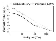
Fig. 6. Char yield obtained from pyrolysis of bio-oil at two final temperatures: 550 °C and 1000 °C - effect of heating rate.
