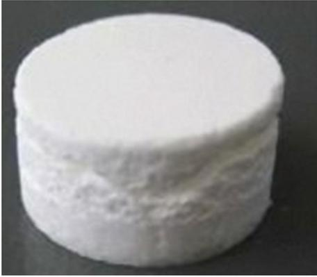
Fig. 20. Capping of a tablet of lactose after ejection.
