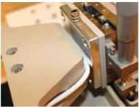
Figure 5: Feeder cable and metallic plane partial discharge set-up
