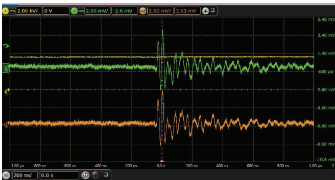
Figure 7: Zoom on partial discharge signal at low pressure (bottom) and atmospheric pressure (top)
