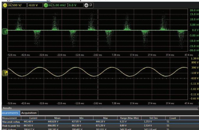
Figure 2: PRPD figure at 100mbar
