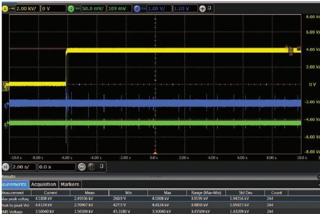
Figure 6: Typical DC discharge behavior 500V above PDIV
