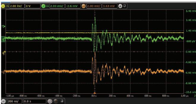
Figure 7: Zoom on partial discharge signal at low pressure (bottom) and atmospheric pressure (top)
