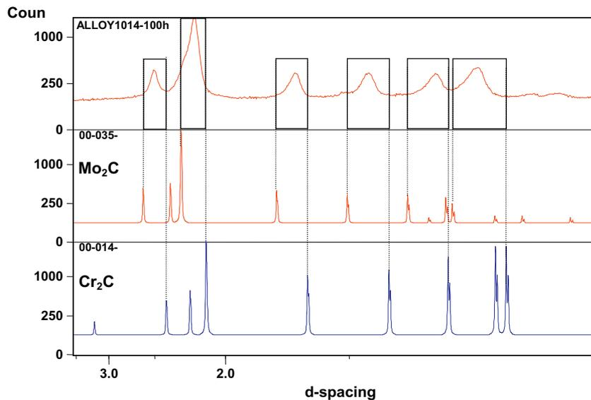
Fig. 3. XRD spectrum for the Alloy1014 grade tempered for 100 h at 500 °C (carbide powder after matrix dissolution). The positions of the peaks correspond to diffraction by hexagonal  $(\text{MoCr})_2\text{C}$  carbide.
