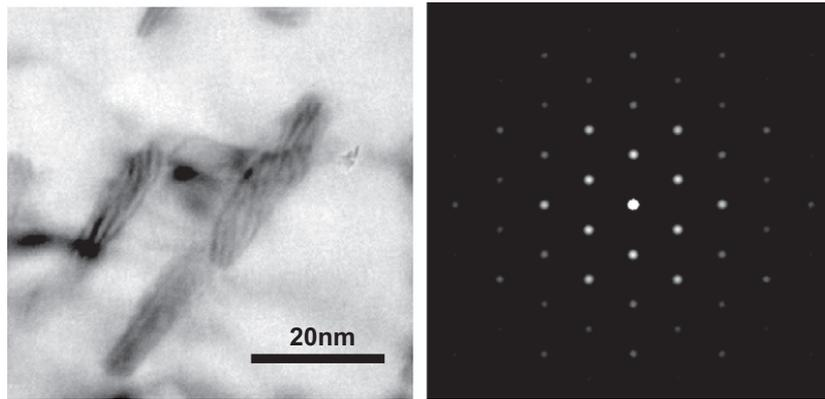
Fig. 4. (Left) Bright field TEM image of  $M_2C$  carbides and (right) the corresponding diffraction pattern for the Alloy1014 grade.
