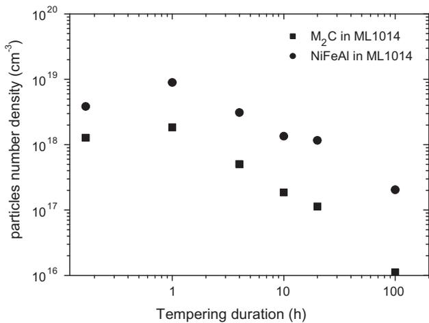
Fig. 12. Comparison of the  $M_2C$  and NiFeAl number densities in the Alloy1014 grade with tempering duration. Data obtained by SANS [18].
