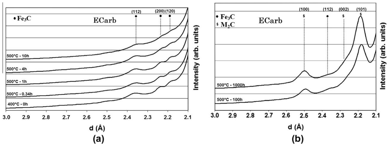
Fig. 5. Synchrotron XRD spectrum for the Ecarb grade for a simple ramp to 400 °C and directly back to room temperature and various tempering times at 500 °C from (a) 0.34 to 10 h and (b) 100 to 1000 h.
