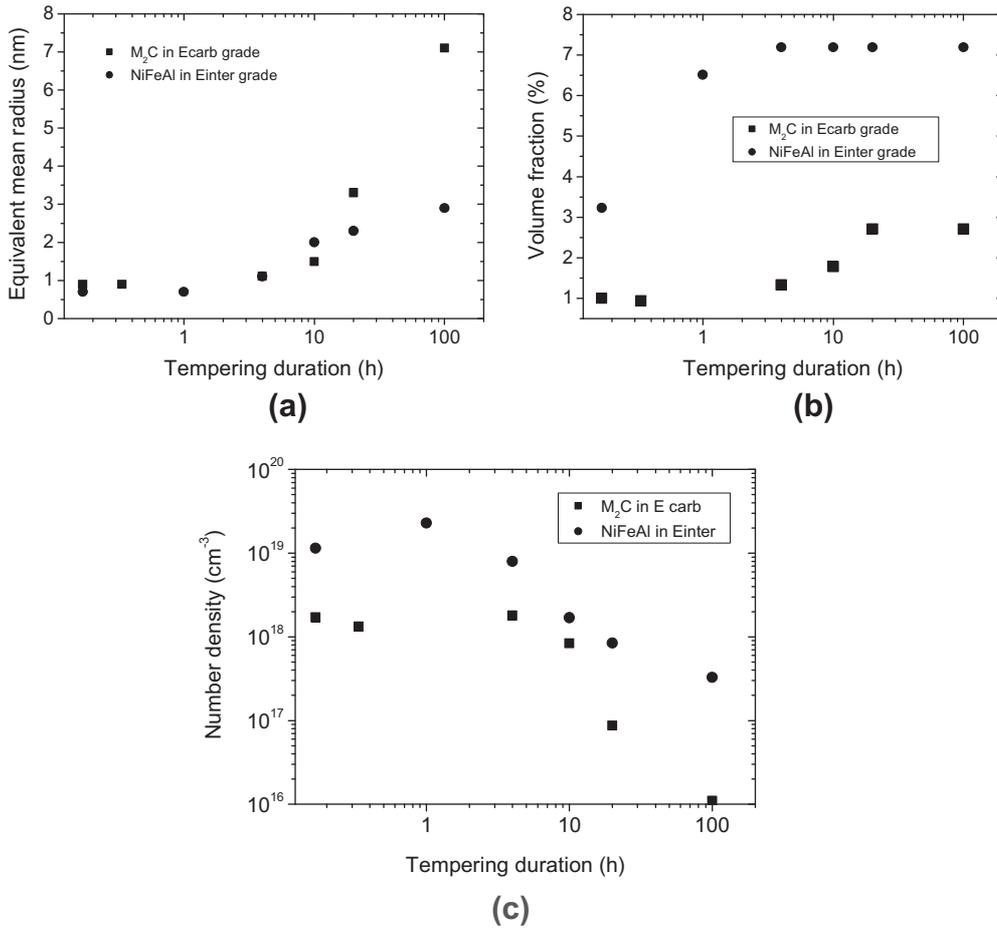
Fig. 10. Comparison of the kinetics of precipitation of FeNiAl and  $M_2C$  particles in the Einter and Ecarb grades: (a) equivalent radius; (b) volume fractions; (c) number densities. Data obtained by SANS [18].
