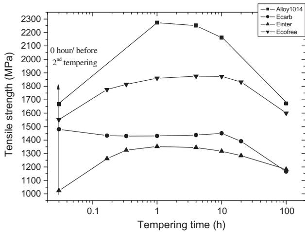
Fig. 2. Tensile strength with tempering time at 500 °C.
