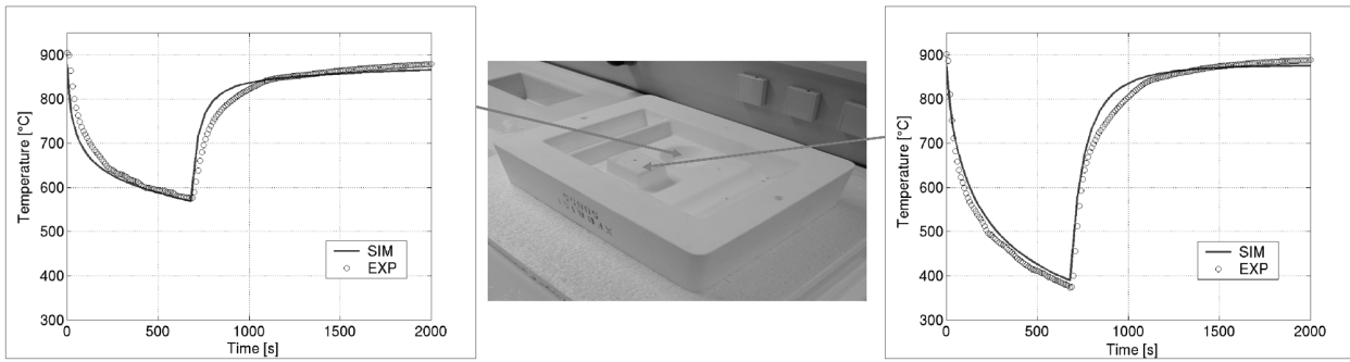
Figure 7. Comparison of experimental and calculated thermal cycles for two different locations at the surface of the ceramic mould (hole and hump).
