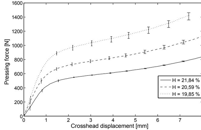
Figure 4: Compression load for three values moisture
