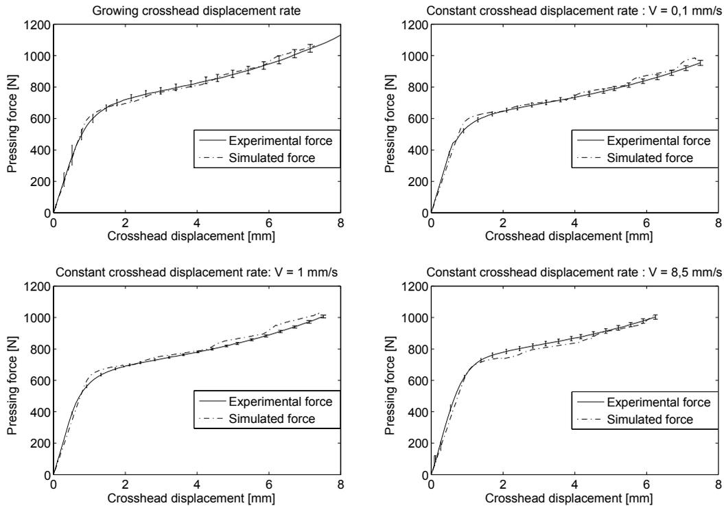
Figure 3: Comparison between the experimental/numerical compression load.
