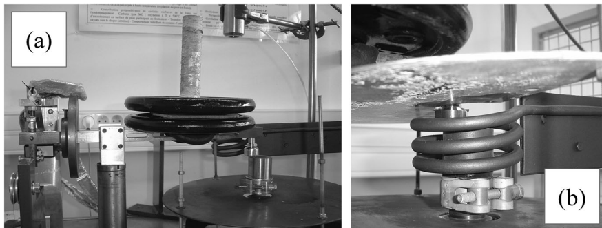
Figure 1. (a) General view of the pin-on-disc tribometer (b) and detail of the inductive heating system.
