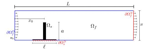
FIGURE 6. Physical setting of the fluid-structure optimization problem of Section 6.2. During optimization, the black domain cannot be reduced but only enlarged by adding reinforcements.
