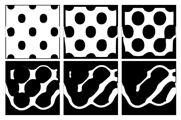
FIGURE 14. From left to right and top to bottom: iterations 1, 15, 30, 110, 220 and 300 of the optimization process in the convective heat transfer of Section 6.3 in the situation (Ex.1).
