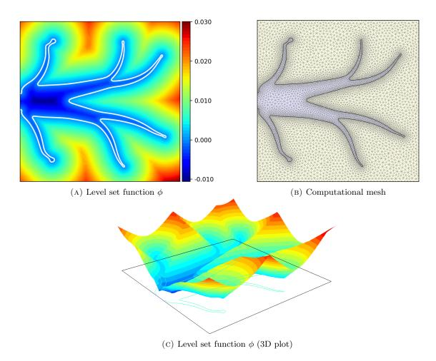
FIGURE 3. Representation of a two-phase partition  $\Omega = \Omega_f \cup \Omega_s$  by means of a level set function on the computational mesh. The fluid-solid interface  $\Gamma$  (the black line on picture (b)) delimits the boundary between the explicitly meshed subdomains  $\Omega_f$  and  $\Omega_s$ .
