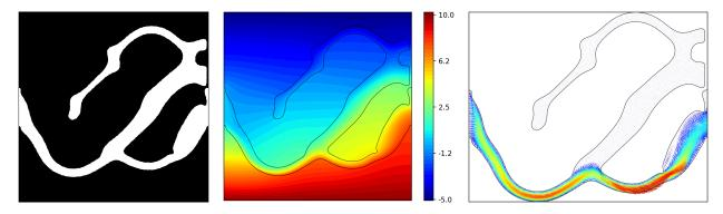
FIGURE 12. Left: optimized configuration for the convective heat transfer test case (Ex.1) of Section 6.3, where the temperature at the upper wall, at the inlet and at the lower wall satisfy  $T_{\rm up} < T_{\rm in} < T_{\rm low}$ . Middle: corresponding temperature field T. Right: fluid velocity field  $\boldsymbol{v}$ .
