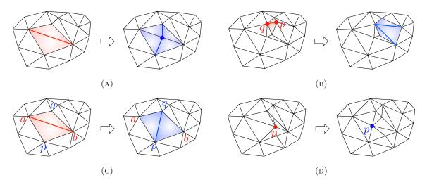
FIGURE 4. Local remeshing operations: (a) split of the red edge by insertion of a new vertex; (b) collapse of the 'small' edge pq; (c) swap of the edge ab for the alternate configuration pq; (d) relocation of point p to improve the quality of the local configuration.
