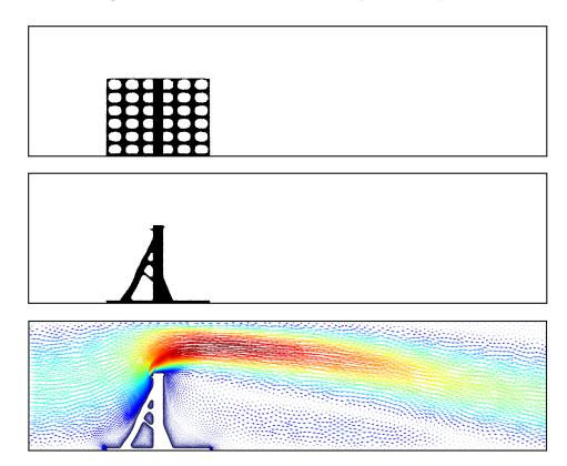
FIGURE 8. Top: initialization. Middle: optimized shape in the fluid-structure example of Section 6.2 (the solid phase is depicted in black); bottom: velocity field v associated to the optimized shape.
