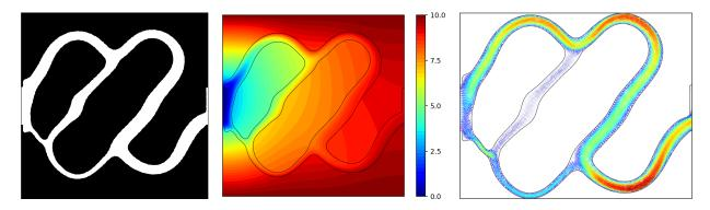
FIGURE 13. Left: optimized configuration for the convective heat transfer test case (Ex.2) of Section 6.3, where the temperature at the upper wall, at the inlet and at the lower wall satisfy  $T_{\rm in} < T_{\rm up} = T_{\rm low}$ . Middle: corresponding temperature field T. Right: fluid velocity field  $\boldsymbol{v}$ .
