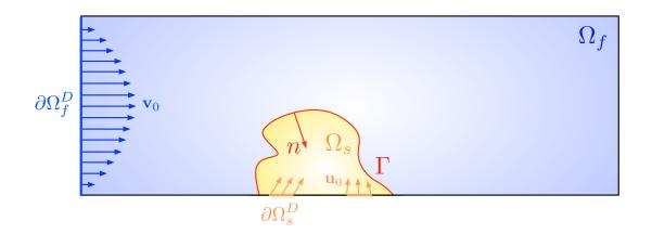
FIGURE 1. Setting of the considered three-physic problem (not all the regions of  $\partial\Omega$  featured in (2.1) (2.2) and (2.3) are represented, see the numerical Section 6 for more complete settings).
