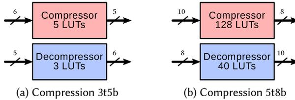
Fig. 9. Compressors and decompressors of balanced ternary values
