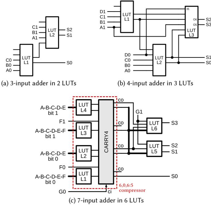
Fig. 7. Optimized implementations of balanced ternary adders
