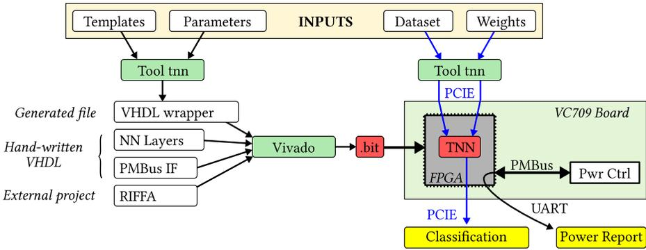
Fig. 11. FPGA demonstrator setup
