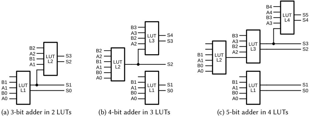
Fig. 6. Optimized implementations of 2-input adders
