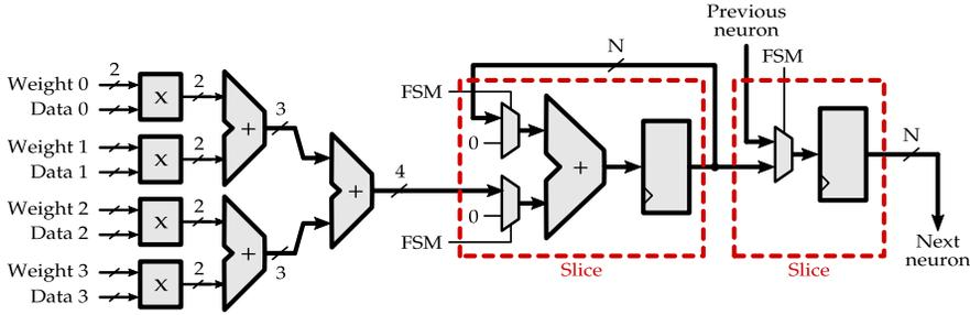
Fig. 4. Neuron implementation, with parallelism degree 4 for input
