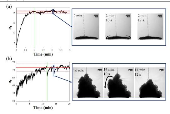
**Figure 2.** Angle of repose evolution over time, with indicated stabilization time  $t_{ss}(|)$ , steady state angle  $\alpha_{ss}(-)$  and cohesiveness  $\sigma_{ss}(\cdot \cdot \cdot)$ . (a) Emulsion stabilized by Krytox (2% wt) where droplets slide off the edge of the support. (b) Fluorinated Pickering emulsion with consecutive avalanches events (all pile images are tilted 180°).
