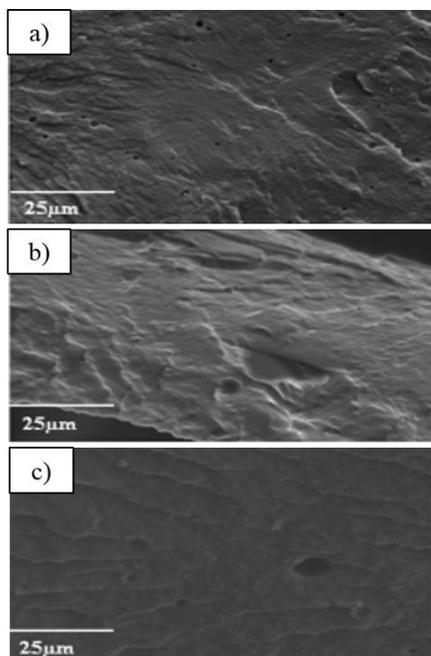
**Figure 18.** Cryofractured SEM micrographs of (a) pure PU, (b) PU with 3 wt% natural talc and (c) PU with 3 wt% Ni-Talc. Reprinted with permission from ref <sup>[112]</sup>.
