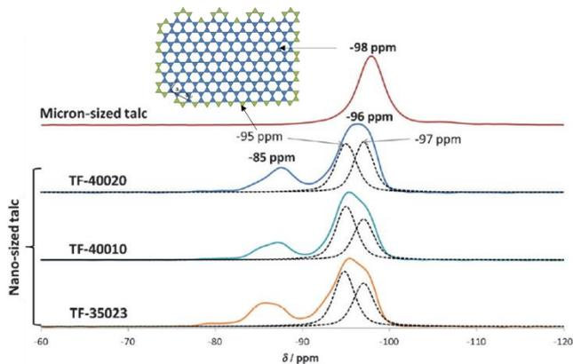
**Figure 14.**  $^{29}\text{Si}$  MAS-NMR spectra recorded on natural talc and synthetic talc. Reprinted with permission from ref [96]. scheme of the talc tetrahedral sheet. Reprinted with permission from ref [65].
