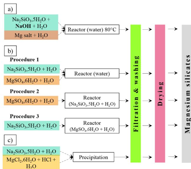
**Figure 20.** Schemes of the procedure followed to synthesize magnesium silicate according to (a) Krysztafkiewicz *et al.*, (b) Ciesielczyk *et al.* and (c) Dietemann *et al.* Reprinted with permission from ref <sup>[123,126,127]</sup>.
