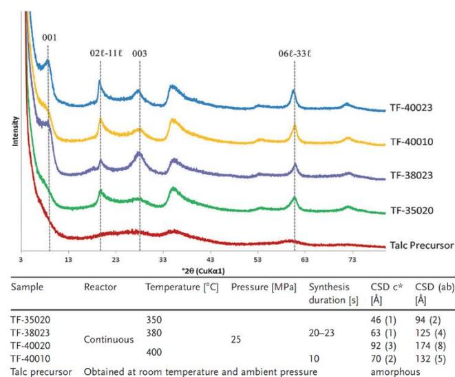
**Figure 11.** XRD patterns of synthetic talc obtained using the continuous near- and supercritical hydrothermal synthesis process for different temperatures (350, 380 and 400°C) and for different synthesis times (10 or 20 seconds). Conditions of synthesis and coherent scattering domain (CSD) measurements. Reprinted with permission from ref [96].
