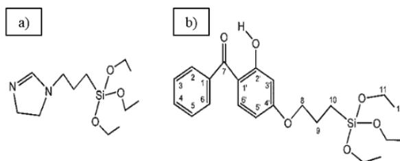
**Figure 29.** Structure of N-(3-triethoxysilylpropyl)-4,5-dihydroimidazole (IM2H) (a) and 2-hydroxy-4-(3-triethoxysilylpropoxy)-diphenylketone (HTDK) (b). Reprinted with permission from ref <sup>[100,106]</sup>.
