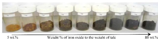
**Figure 19.** Magnetic synthetic talc ranges obtained. Reprinted with permission from ref <sup>[65]</sup>.
