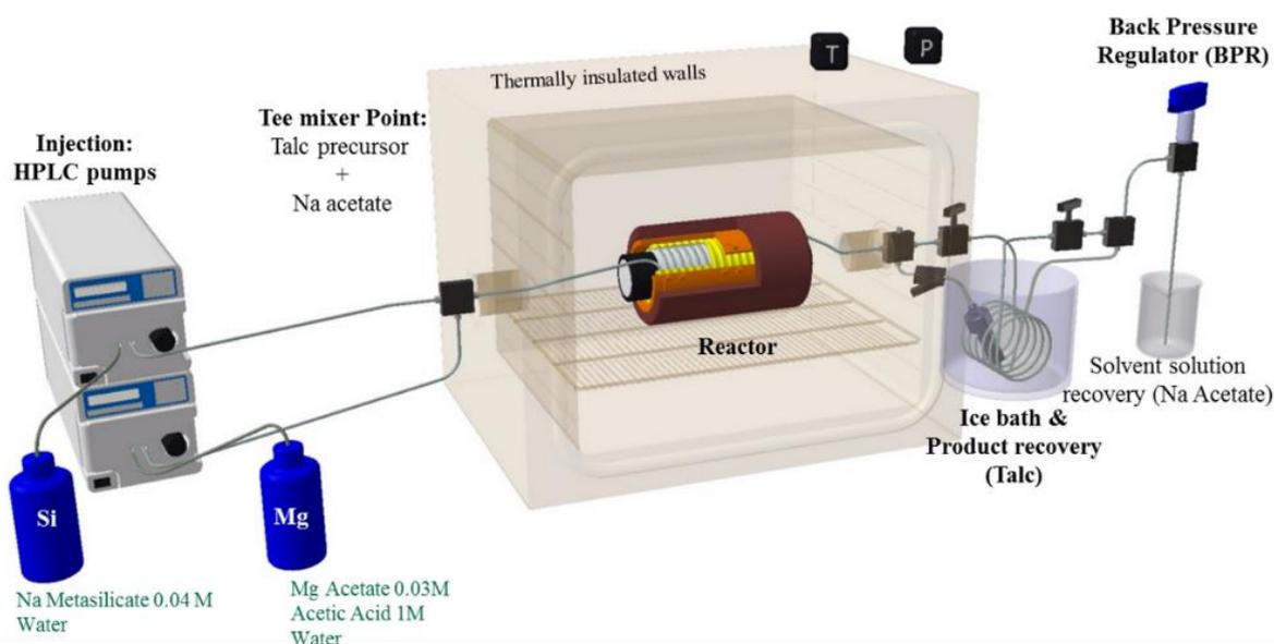
**Figure 10.** Custom-built continuous supercritical hydrothermal process for talc synthesis. T = thermocouple; P= manometer. Reprinted with permission from ref <sup>[96]</sup>.
