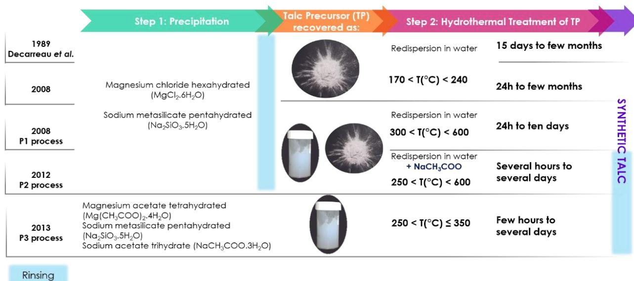
Figure 4. Evolution of the hydrothermal talc synthesis process. Reprinted with permission from ref <sup>[56]</sup>.
