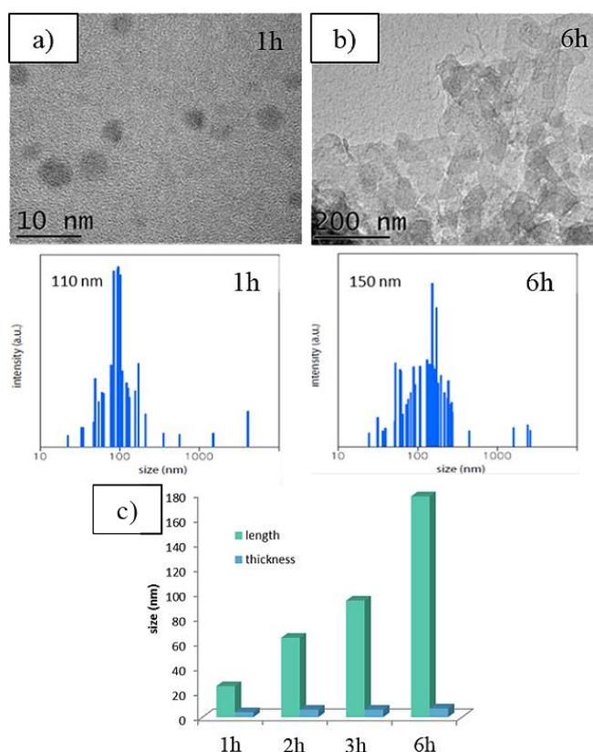
**Figure 12.** TEM images and size distribution histogram analysis of synthetic talc after (a) 1h and (b) 6h of hydrothermal treatment and (c) evolution of the length and the thickness of particles with synthesis duration (estimated from low-pressure adsorption analyses). Reprinted with permission from ref [65].
