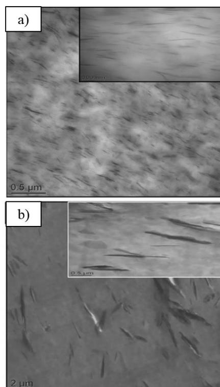
**Figure 17.** TEM micrographs of (a) PA6/synthetic talc and (b) PA6/natural talc. Reprinted with permission from ref <sup>[108]</sup>. This figure shows a higher exfoliation and dispersion of synthetic talc in the matrix in comparison with natural talc.
