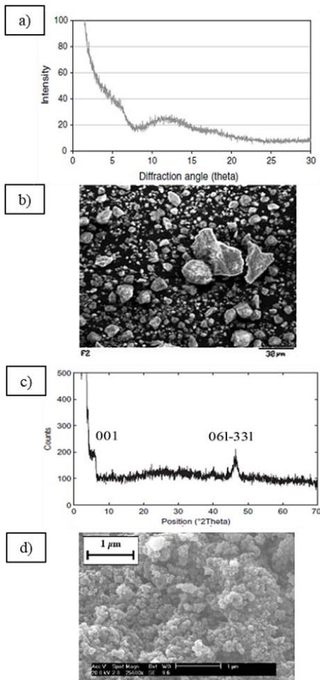
**Figure 21.** (a) XRD and (b) SEM micrographs of synthetic magnesium silicate obtained by Ciesielczyk *et al.* and (c) XRD and (d) SEM micrographs of synthetic magnesium silicate obtained by Dietemann *et al.* Reprinted with permission from ref [125,127].
