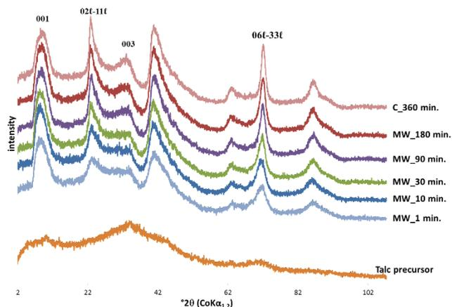
**Figure 8.** XRD patterns of synthetic talcs obtained by microwaves (MW) heating at 230 °C under autogenous vapor pressure for synthesis time varying between 1 to 180 minutes. MW-talc samples are compared to a talc precursor and synthetic talc obtained using a conventional heating system at 230°C for 360 minutes. Reprinted with permission from ref [65].
