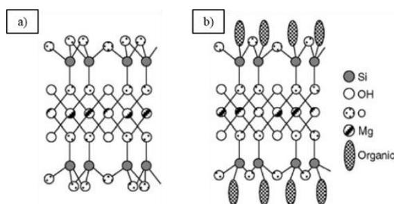
**Figure 23.** (a) TOT layer structure of a natural talc and (b) Proposed TOT layer structure of an organotalc. Reprinted with permission from ref <sup>[137]</sup>.
