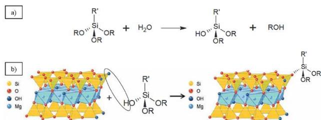
**Figure 27.** (a) Organoalkoxysilane hydrolysis and (b) condensation with talc. Reprinted with permission from ref <sup>[100]</sup>.
