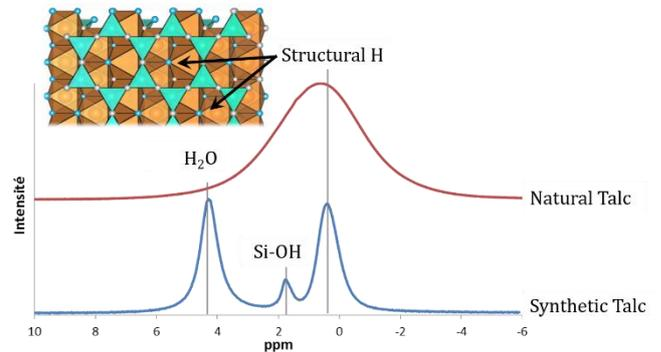
**Figure 15.**  $^1\text{H}$  MAS-NMR spectra recorded on natural talc and P3-synthetic talc. Reprinted with permission from ref [65]. Scheme of the talc layer (top view).
