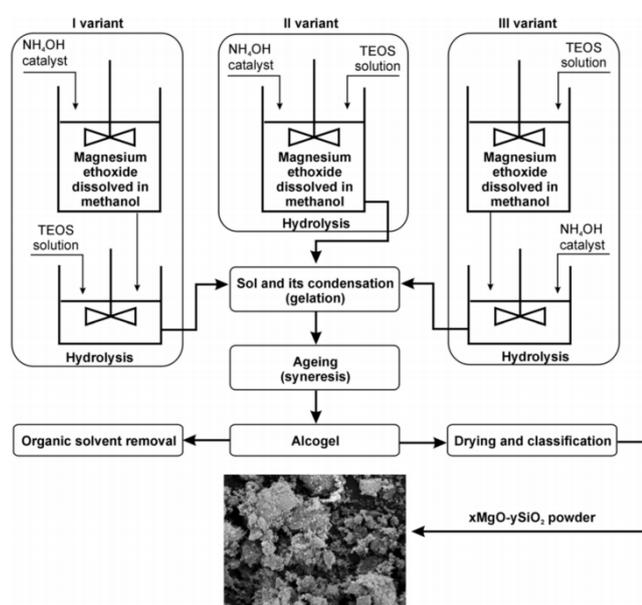
**Figure 25.** Methodology of precipitation of  $x\text{MgO}\cdot y\text{SiO}_2$  powders ( $0.64 \leq x \leq 0.99$  and  $0.83 \leq y \leq 1.00$ ) via the sol-gel method according to Ciesielczyk *et al.* Reprinted with permission from ref <sup>[165]</sup>.
