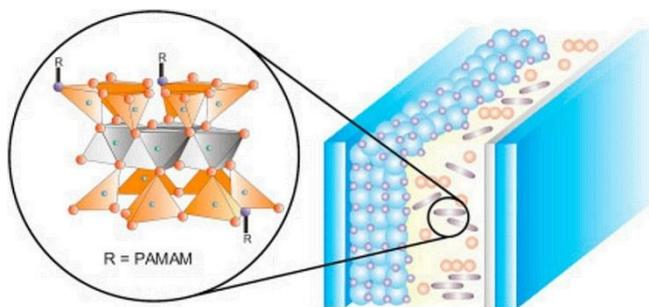
**Figure 26.** Scheme showing dendron-modified talc to gel liquid electrolytes and apply to dye-sensitized solar cells. Reprinted with permission from ref <sup>[173]</sup>.
