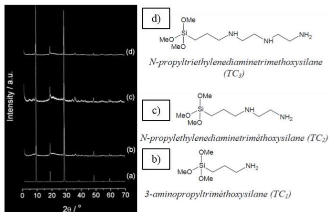
**Figure 28.** XRD of (a) talc and grafted talc using (b) TC<sub>1</sub>, (c) TC<sub>2</sub> and d) TC<sub>3</sub>. Reprinted with permission from ref <sup>[181]</sup>.
