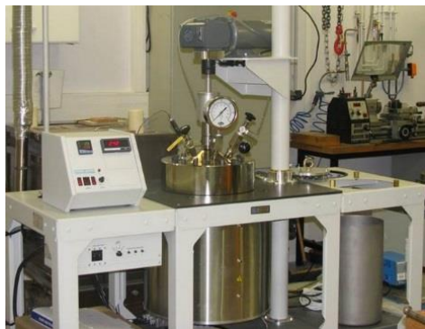
Figure 5. A 18.5L stainless steel autoclave used for the preparation of P3-nanotalc (GET laboratory, Toulouse, France; Parr Instrument Company; property of Imerys Talc Europe).
