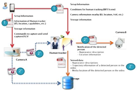
Fig. 3. Data flow schematics of a city video surveillance system
