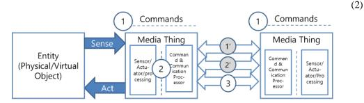
Fig. 1. Conceptual architecture of IoMT standardization
