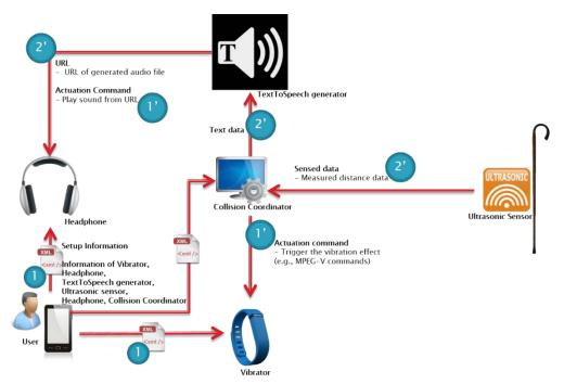
Fig. 5. Data flow schematics of a blind pedestrian collision aviodance system
