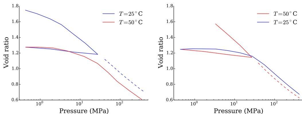
**Figure 2. Consolidation test on clay interrupted by temperature changes after unloading, adapted from Habibagahi (1977). This result proves that temperature has an impact on preconsolidation pressure, even if no irreversibility occurs during the change of temperature. (left) Case of an increase of temperature: the preconsolidation pressure decreases. (right) Case of a decrease of temperature: the preconsolidation pressure increases.**
