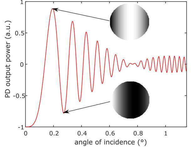
Fig. 3: Simulation of the OFI signal for a rotation of the sensor by  $1^\circ$  with a laser spot of diameter  $60 \mu\text{m}$ . The circle plots represent the distribution of phases of the backscattered wave re-entering the laser cavity over the laser spot on the target at two different aperture angles.
