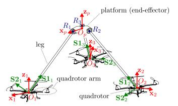
Fig. 1: A flying parallel robot with three quadrotors
