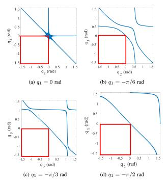
Fig. 4: Singularity locus ( $|\det \mathbf{A}| < 5\mathrm{e}{-4}$ ) for the passive architecture with  $\ell_{O_pR_i} = 0.1$  m and  $\ell_{R_iO_i} = 0.8$  m. The red square areas represent a singularity free workspace.
