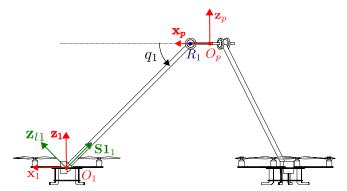
Fig. 2: Side view of the flying parallel robot
