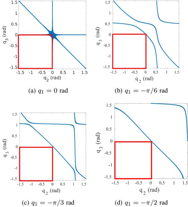
Fig. 4: Singularity locus ( $|\det \mathbf{A}| < 5e-4$ ) for the passive architecture with  $\ell_{O_p R_i} = 0.1$  m and  $\ell_{R_i O_i} = 0.8$  m. The red square areas represent a singularity free workspace.
