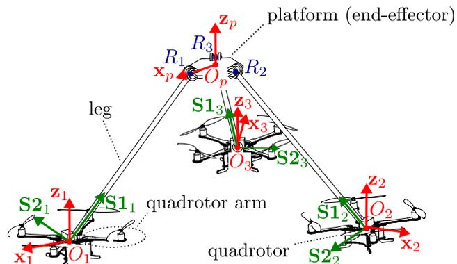
Fig. 1: A flying parallel robot with three quadrotors
