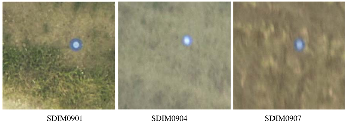
Fig. 18. Zoomed detail of 20 mm resolution images for sharpness assessment (the blue objects are geo-referencing targets of 30 mm diameter distributed around the crop field)
