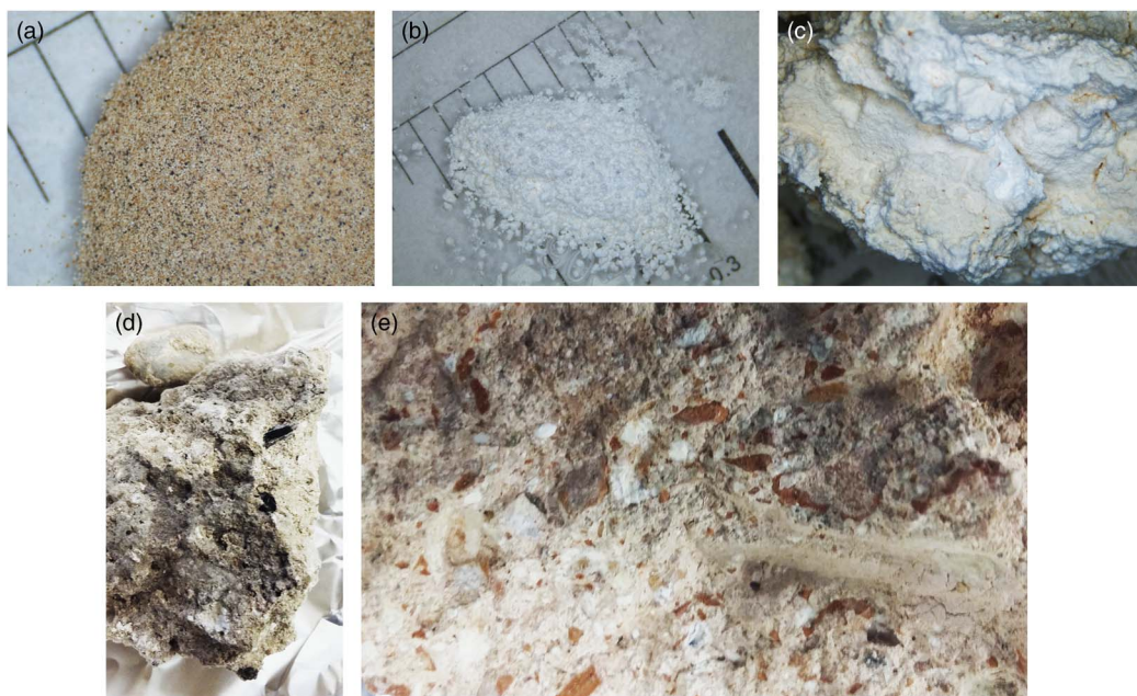
Figure 1 Pictures of MODIS samples distributed among the laboratories: (a) Sample 1—Finnish mortar; (b) Sample 2—Mallorca lime burial f < 500 \mu m; (c) Sample 2—Mallorca lime burial original (F); (d) Sample 3—Basel mortar; (e) Sample 4—Roman cocciopesto.
