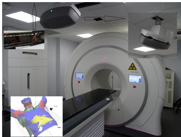
FIG. 1. Catalyst camera in the TomoTherapy room. The camera is attached to a rail on the ceiling to facilitate maintenance of the TomoTherapy machine. Lower left inset: view of the live (blue) and reference (green) contours. The red and yellow zones are also projected live on the patient, representing regions that are too much anterior (red) or posterior (yellow). This example shows a pitch issue with the patient and the breast board.
