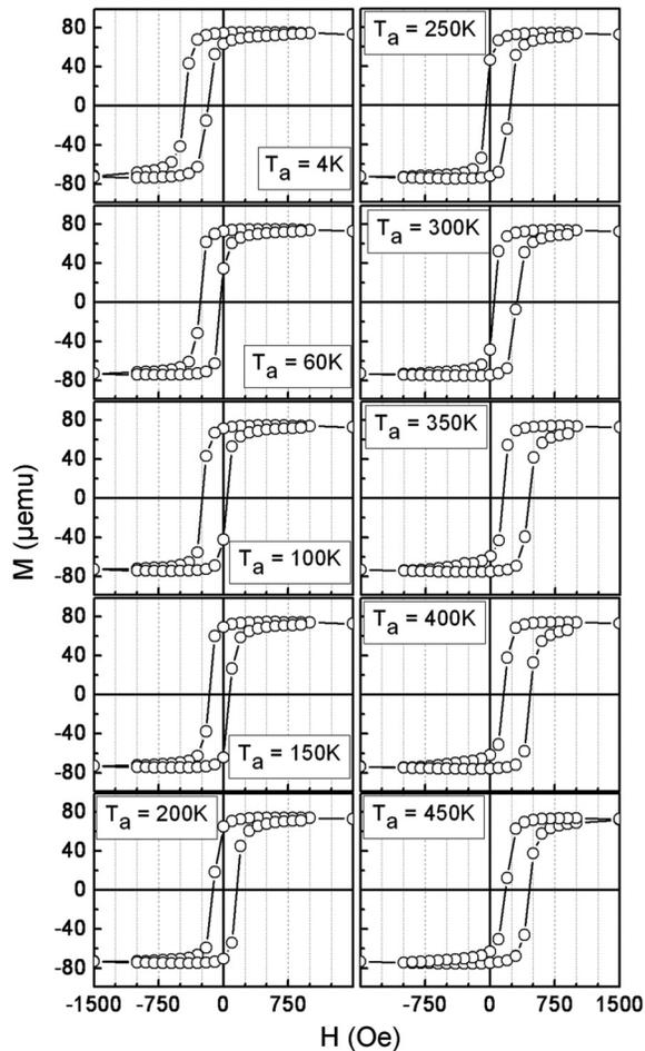
FIG. 1. Representative hysteresis loops measured by SQUID at 4 K along the field cooling (FC) direction, for different annealing temperatures ( $T_a$ ), for a film of Ta (3 nm)/Cu (3 nm)/Co (3 nm)/Pt (1 nm)/IrMn (3.8 nm)/Pt (2 nm). The loops are subsequent to a specific cooling procedure: the samples were initially FC under a positive saturating field of 10 kOe from 450 K down to 4 K.  $T$  was then raised up to  $T_a$  and the samples were FC under  $-10$  kOe from  $T_a$  down to 4 K.
