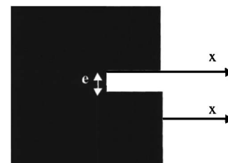
FIG. 9. Schematic upper view of a square down-down (black) magnetized domain with a nonreversed channel of width “e.” The distance x is taken either from the square side or the base of the channel.
