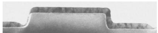
Fig. 5. TEM image ( 457\ \text{nm} \times 370\ \text{nm} ) of a \text{Pt}_{1.8\text{nm}}(\text{Co}_{0.6\text{nm}}/\text{Pt}_{1.8\text{nm}})_4 multilayer deposited on a 150/100/36 line array.
