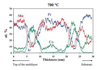
FIG. 6. Pt, Co, Ir, and Mn concentration profiles related to  $[(Pt/Co)_3/IrMn]_7$  multilayered samples annealed at  $700\,^{\circ}$ C.
