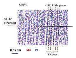
FIG. 5. APT elemental maps showing the distribution of Pt and Mn atoms in the PtMn region (see Fig. 3) of [(Pt/Co)<sub>3</sub>/IrMn]<sub>7</sub> multilayered samples annealed at 500 °C. (111) atomic planes containing both Pt and Mn atoms are imaged.
