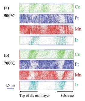
FIG. 4. APT elemental maps showing the distribution of Pt, Co, Ir, and Mn atoms in  $[(Pt/Co)_3/IrMn]_7$  multilayered samples annealed at 500 and 700 °C.
