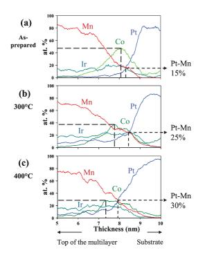
FIG. 3. Concentration profiles related to Pt, Co, Ir, and Mn atoms at the  $\text{Co}_{(3)}$ /IrMn interface of three  $[(\text{Pt/Co})_3/\text{IrMn}]_7$  multilayered samples before and after annealing at 300 and 400 °C.
