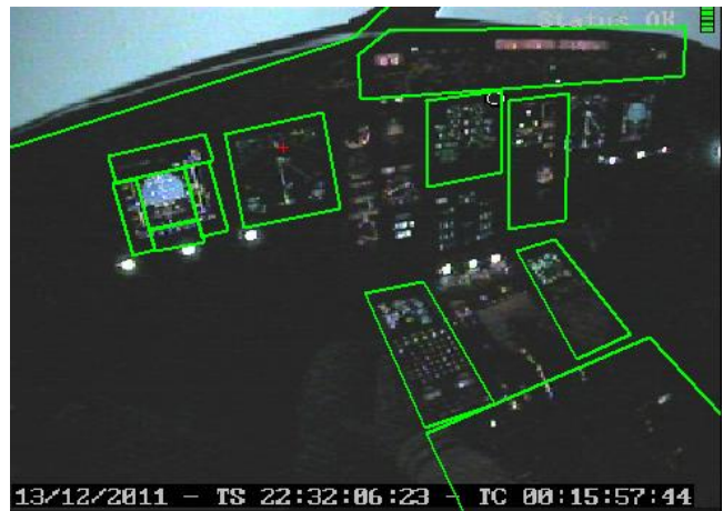
Figure 2 — Example of Captain's AOIs delimiting flight deck instruments (Airbus A330).
