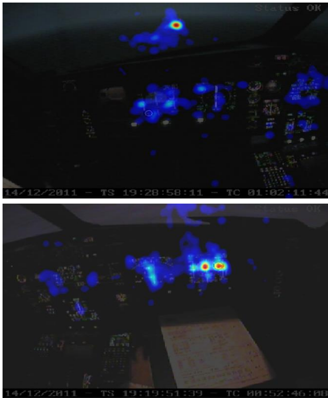
Figure 1 — Heatmaps examples of a Captain when he is PM (on top) and a First Officer when he is PF (at the bottom), between 1500 and 500 ft (the two pictures come from an Airbus A330 cockpit). The 'hot' zones where the users focused their gaze with a higher frequency are indicated by yellow/red colors whereas less attended zones are depicted in dark/blue colors.
