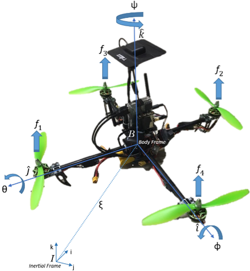
Fig. 2 The Quadrotor aircraft frames scheme
