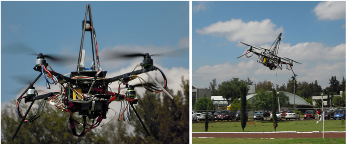
Fig. 15 The Quadrotor aircraft flying at a particular altitude using integral sliding mode control autonomously
