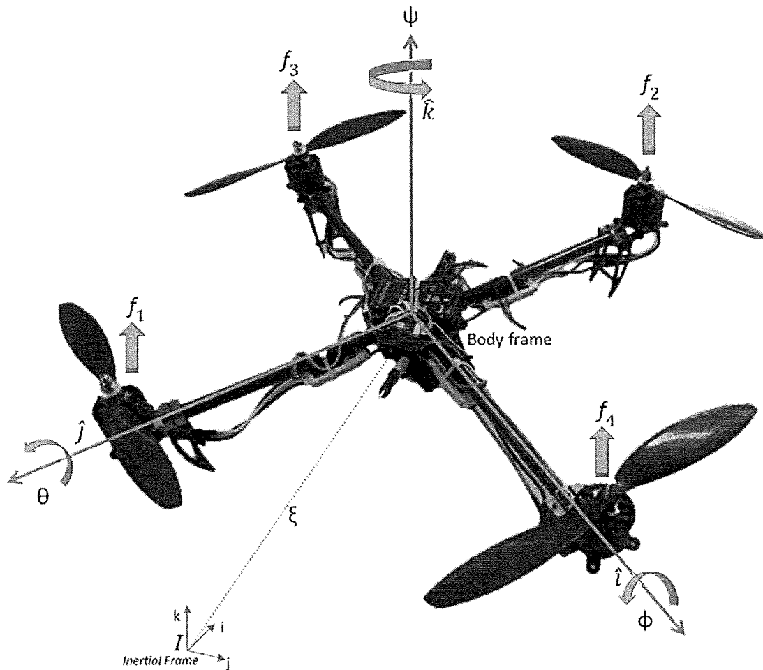
Fig. 1 Scheme of forces produced by rotors, and torques generated in attitude (roll, pitch and yaw angles) acting on the quadrotor
