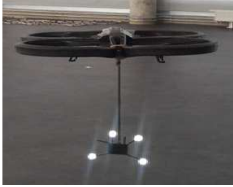
Fig. 1. Experimental platform for a quadrotor with a cable-suspended payload.
