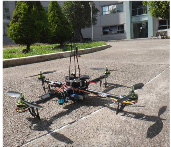
Fig. 1: Photo of the Quadrotor aircraft used with the embedded control system pixhawk .
