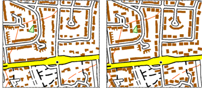
Figure 14: Derivation of the 1:25k topographic map (right) from the BD TOPO ® database (left, 1m resolution) at IGN-France.
