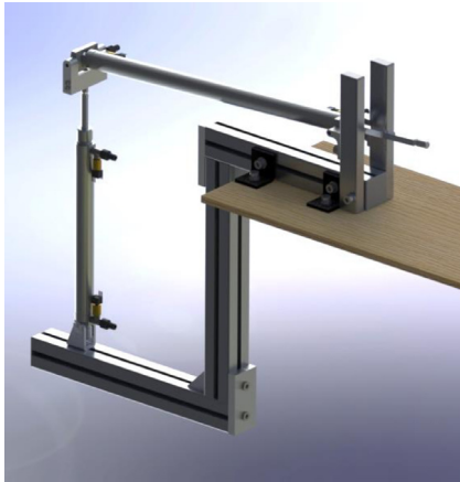
Fig. 1. 2 DOF actuated pneumatic haptic interface.
