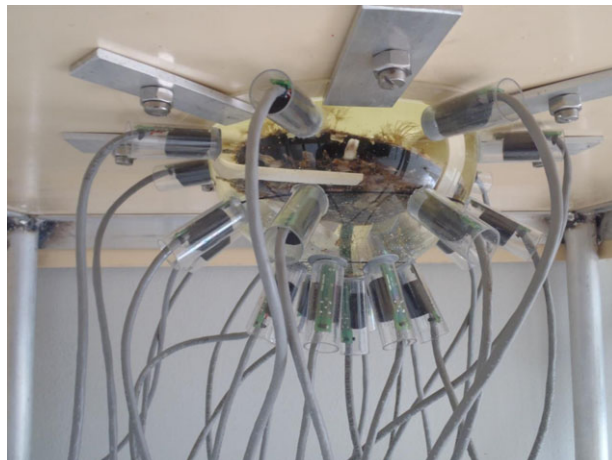
Figure 2. Overview of the magnetometer system. For data acquisition, the grafted pearl oyster Pinctada margaritifera is placed into the dome. The movements of a magnetic homemade nucleus (electronic supplementary material, figure S1) inserted in the gonad of a pearl oyster are registered through magnetic field variations measurement with the 25 magnetic sensors located on the convex surface of the dome. The frequency of acquisition is every half-second with a recording periodicity equal to 1 min. Time of acquisition varied from one day to one week. Above the dome, the tank is filled with an open circuit of seawater with the grown microalgae Isochrysis galbana (concentration 1500–4000 cells ml -1 ) to feed the oyster at a constant flow of 10 ml min -1 .
