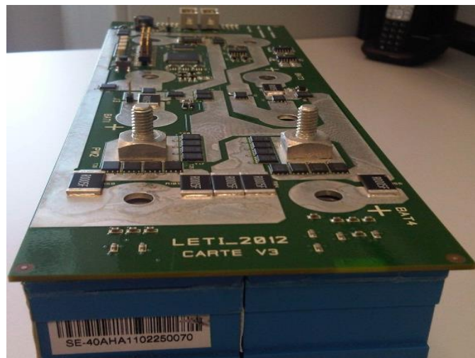
Figure 10 : Picture of the second prototype switched module
